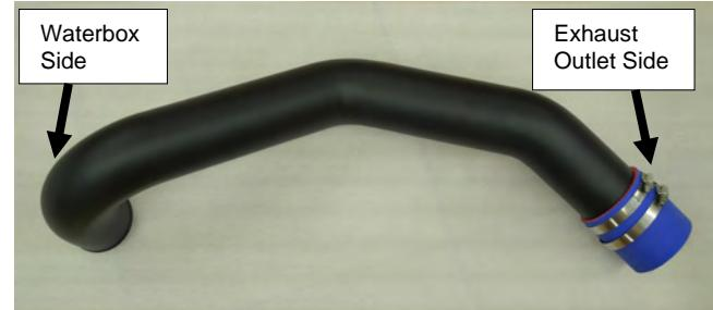
Install exhaust outlet side of tube (side with coupler) onto rear exhaust outlet inside hull. Slide 2nd hose clamp down coupler & into position on outlet. Secure coupler onto outlet with clamp. **Note: Do not over tighten clamp.**
