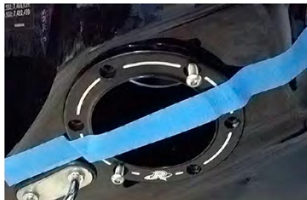
From inside of hull, carefully place supplied billet collar onto exhaust outlet. Ensure raised stand offs are toward the hull.
