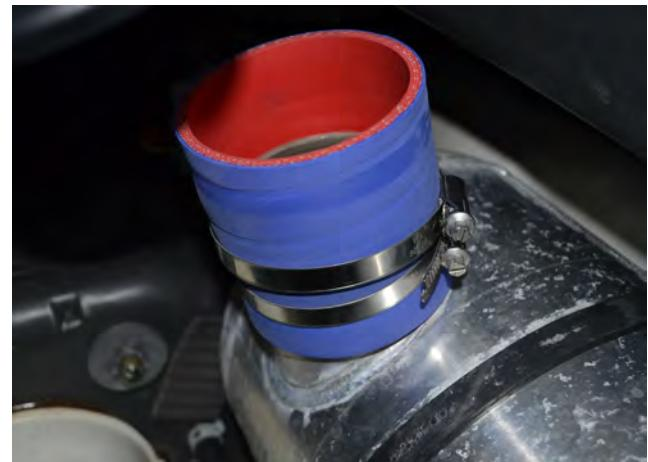
Install supplied coupler onto outlet end of supplied rear exhaust pipe. Secure using supplied hose clamp. **Note: Do not over tighten clamp.**
