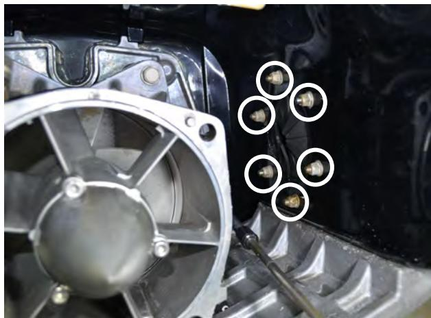
Place supplied billet exhaust outlet block-off onto stock exhaust collar so that raised side of block-off faces the same direction as the six threaded studs. Install supplied rubber gasket over studs and onto billet block-off (adhesive side first).
